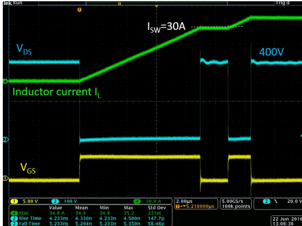
Figure 16 400V/30A double pulse test waveform
